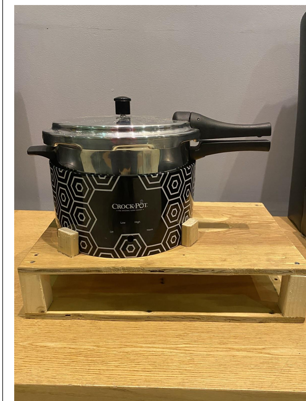
Figure 2: Physical mockup that provided insight on the end users interaction and appropriate dimensions for the hybrid pressure cooker
