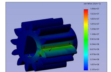
Figure 4: Pinion Gear FEA Model
