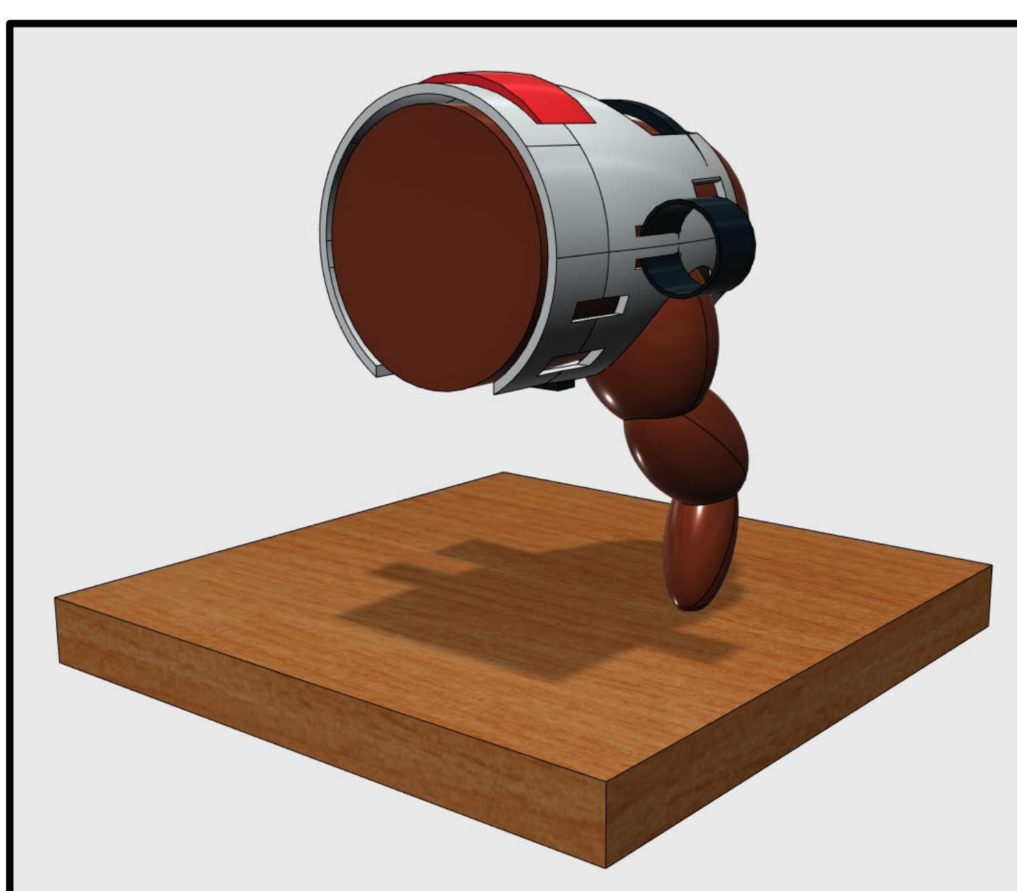
Figure 3: Prototype 2 used a rigid plastic shell as a foundation to build a prosthetic leg off of
