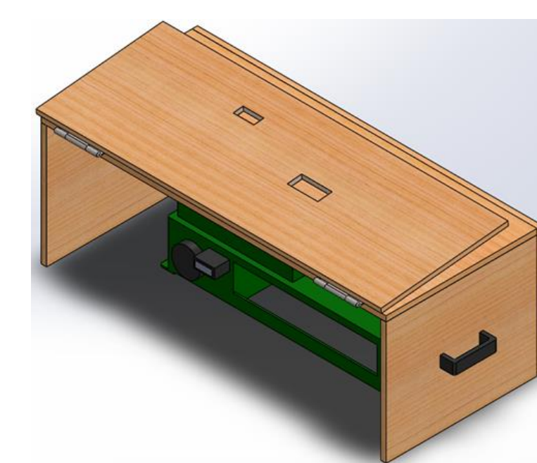
Figure 3: Second design with single set of hinges on back of chamber. Difficulty opening due to door shape/size
