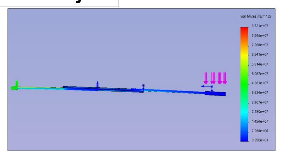
Solidworks Finite Element Analysis (FEA) of the linear slide mechanism. A factor of safety of 3 was obtained.
