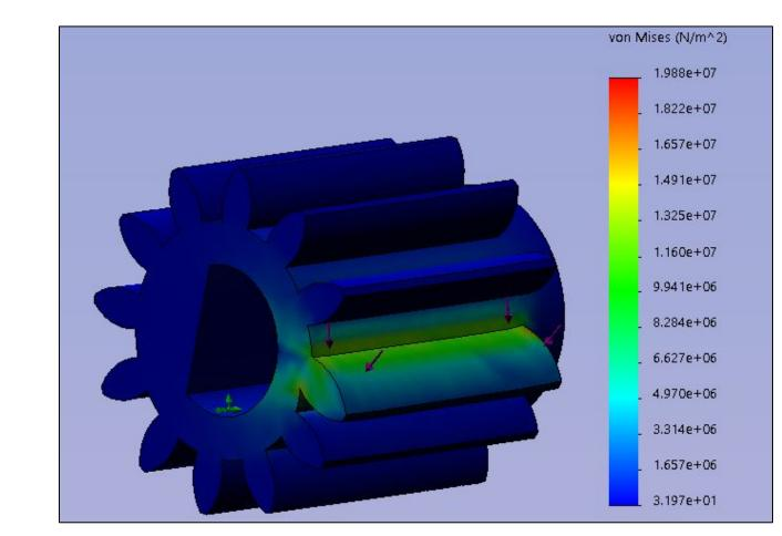
Figure 4: Pinion Gear FEA Model
