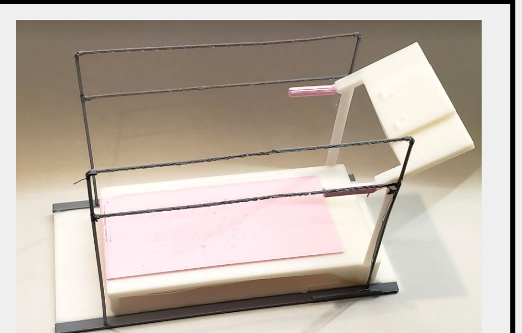
Figure 6: 3D printed 1:10 scale model of the modified treadmill
